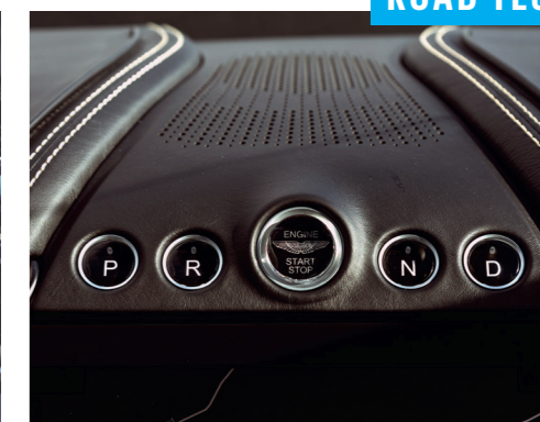
● Aston continues its long-held tradition of individual drive selector buttons. They look great and remove the need for a flimsy column stalk shifter.
