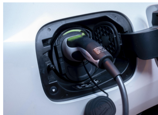
■ A 10-80% charge via a rapid 110kW charger will take just 40 minutes
