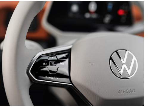
■There is no central gearstick – the ID.3 has side-mounted selectors
