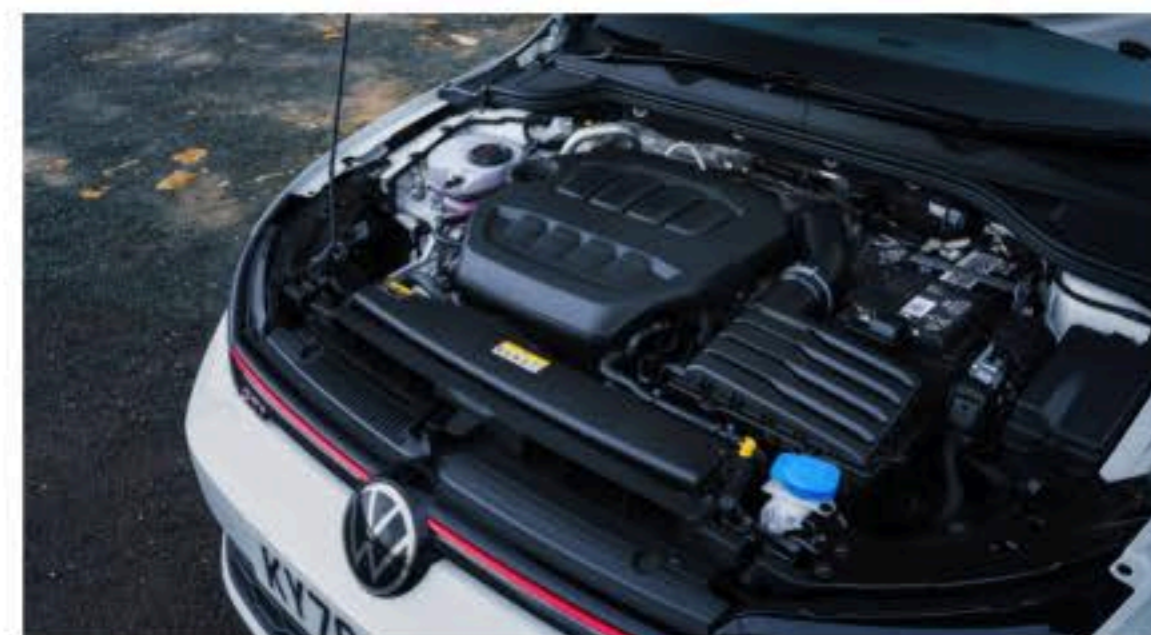
■ The Golf GTI utilises a familiar 2.0-litre turbocharged petrol engine
