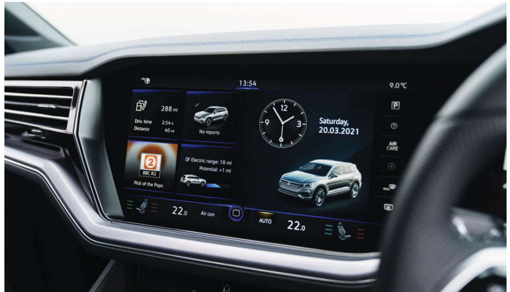
■ A 12-inch digital cockpit, as well as displaying features such as speed and revs, showcases remaining electric charge and charging times
